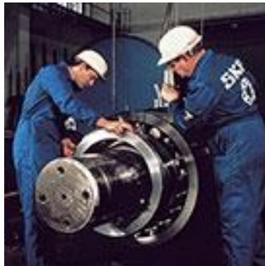
Around 16% of all premature bearing failures are a result of poor fitting or using incorrect mounting techniques. Individual applications may require mechanical, heat or hydraulic mounting methods for correct and efficient bearing mounting. SKF offers you the services for mounting/dismounting technique appropriate for your application which will help you extend your bearing's service life and reduce costs resulting from premature bearing failure as well as potential damage to the application.
